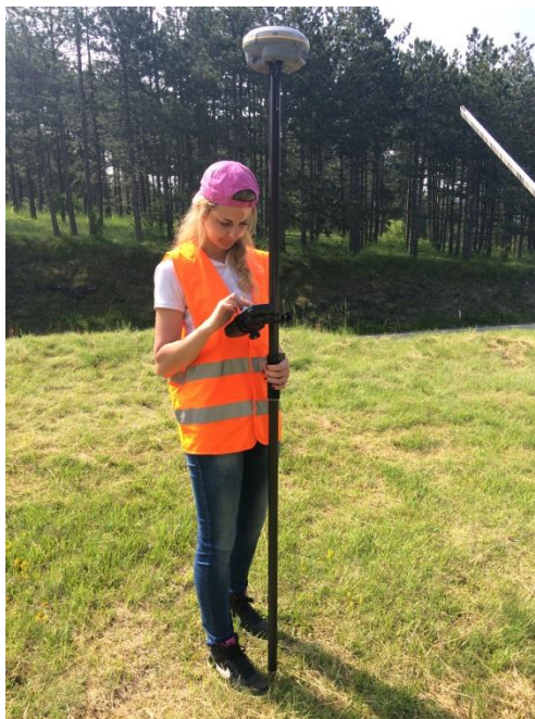
Fig. 3 GNSS RTK using the total station Trimble R8 GNSS at the field practice in Zlatibor mountain
